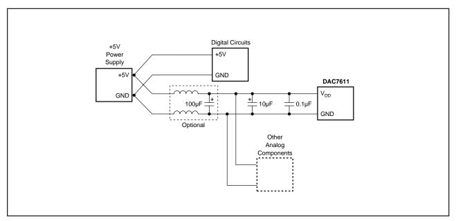
FIGURE 4. Suggested Power and Ground Connections for a DAC7611 Sharing a +5V Supply with a Digital System.
