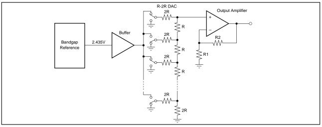
FIGURE 2. Simplified Schematic of Analog Portion.
