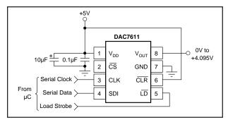
FIGURE 1. Basic Operation of the DAC7611.
