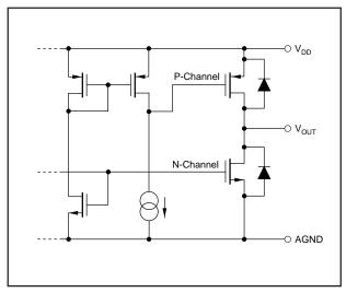
FIGURE 3. Simplified Driver Section of Output Amplifier.
