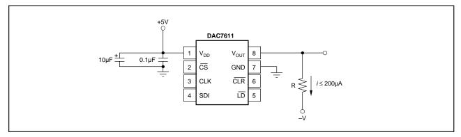
FIGURE 5. Offset Error Measurement Circuit.
